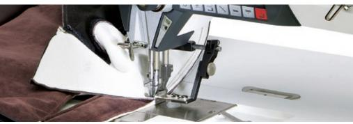
Closing seams/assembly seams during pre-assembly work in the automotive industry
