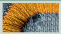
A needle point which is too sharp will create loop damage or needle cuts. A needle, which is too thick will push out the loop under tension and break it.
